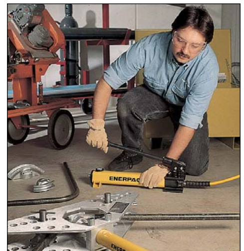
▲ Steel pipe is quickly and safely bent up to 90° using the STB-101H Pipe Bender Set.
