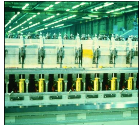
This paper mill uses RD cylinders for precision when trimming. ►
