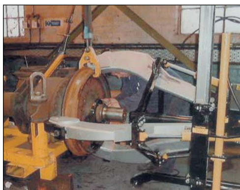
◀ The EPH-1003 quickly and easily removes this drive sheave from its shaft.
