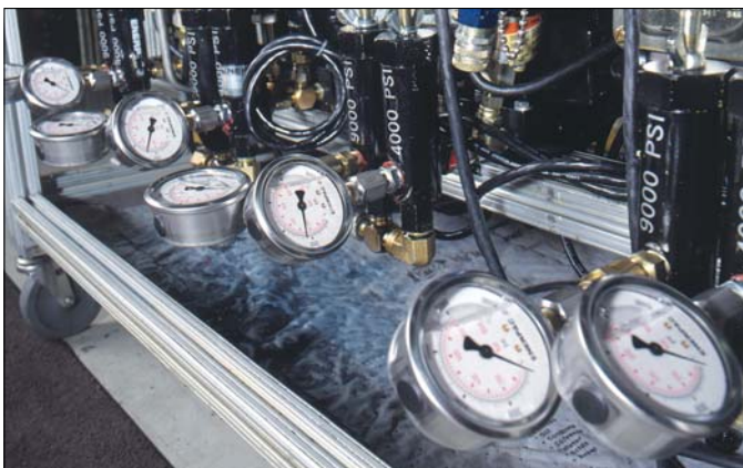
◀ Enerpac glycerine filled gauges, used to cycle test hydraulic pumps in a test lab environment.
