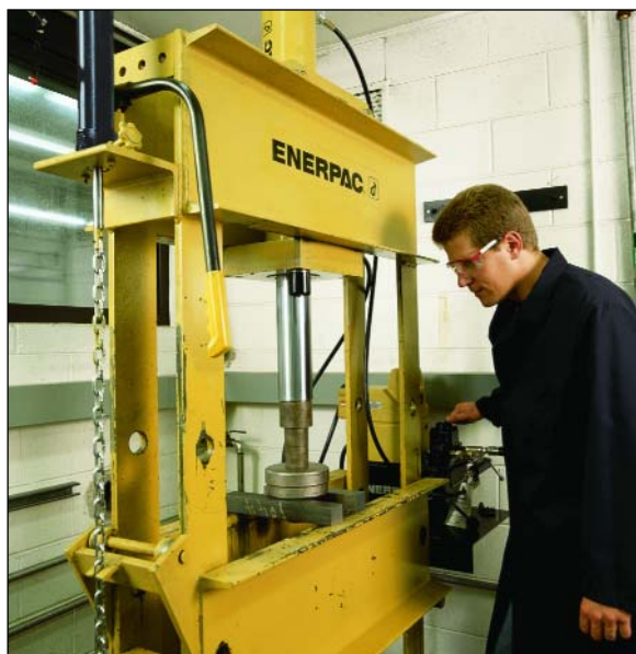
◀ An Enerpac H-Frame press makes quick work of removing the shaft from this assembly.
