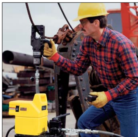
◀ A Titan PUJ-3309E is used with a hydraulic cutter to cut wire rope.
