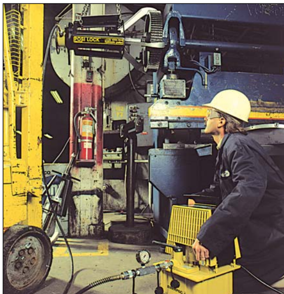
◀ An EPHR-116, 50 ton hydraulic Posi Lock® puller easily removes the main drive gear from this metal forming brake press.
